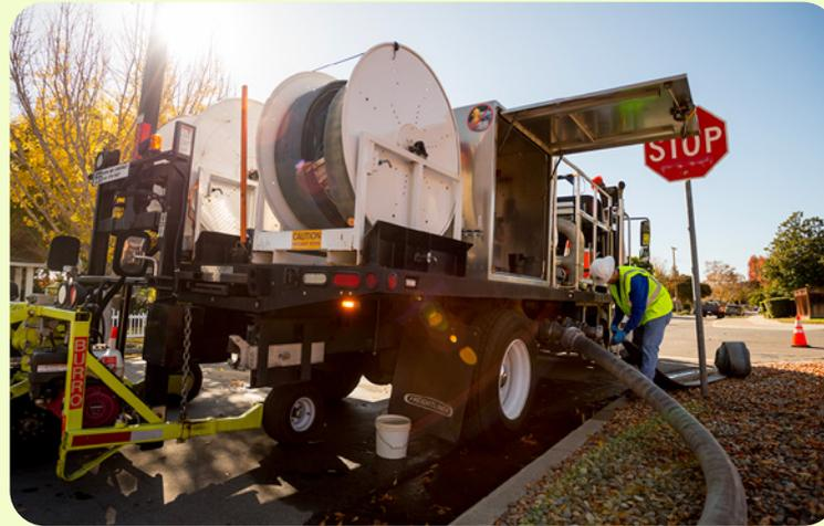
**Flushing Truck** – SJW’s **flushing truck** saves about 30,000 gallons of water per flush compared to traditional flushing methods. That is a savings of approximately 6 million gallons per year. Using Neutral Output Discharge Elimination System (NO-DES) technology, effective flushing and sediment removal is obtained with minimal water waste. SJW is improving water quality while saving water.
